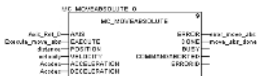
MFB: Programming a movement in absolute mode
