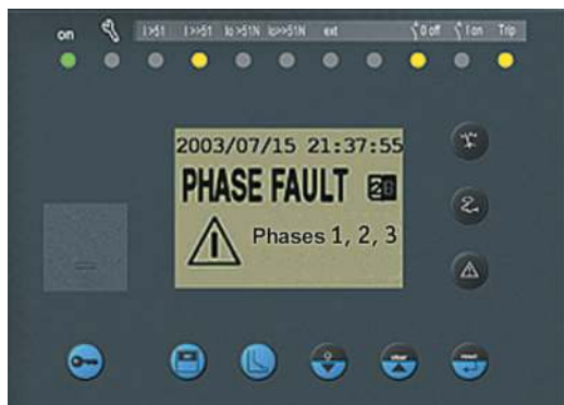
Local indications on the Sepam front panel.
