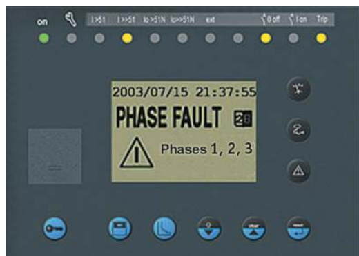
Local indications on the Sepam front panel.
