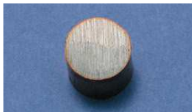
Cu-Bond Round Conductor cross-section
