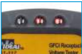
Red Lights Indicate Incorrect Wiring
