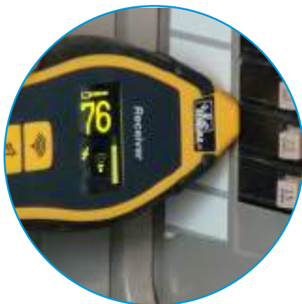
Finding Breakers or Fuses
