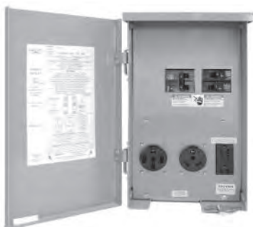
CESMPSC75GRHR NEMA 5-20R2 GFCI, TT-30 travel trailer receptacle, NEMA 14-50. Breakers: 1P 20A, 1P 30A, 2P 50A.
