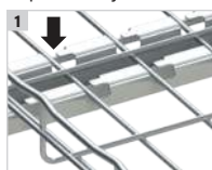
Insert tray into slots
