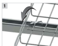
Hook one side of the FS41 into channel support.
